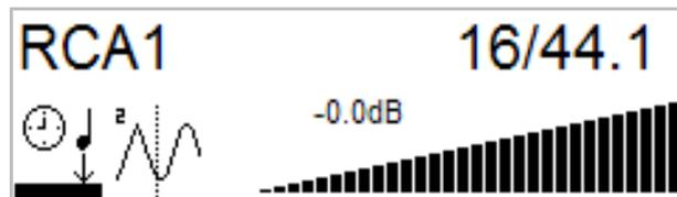
The icons at the bottom left corner are the **Sync** mode (slave to **Audio** is shown) and the selected **Filter** (**Filter 2** is shown). The **Phase** icon appears here if set to inverted.
